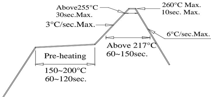
3.2 Reflow soldering should not be done more than two times.
