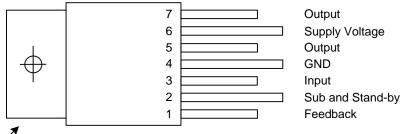
ZTAB Connected to Pin 4
