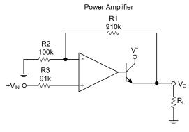
$V_0 {=} 0 \ V_{DC}$  for  $V_{IN} {=} 0 \ V_{DC}, \ A_V {=} 10$
