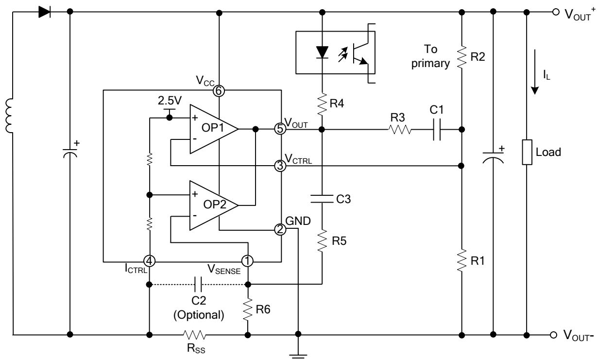
$$V_{OUT} = V_{REF} \times \frac{R1 + R2}{R1}$$
