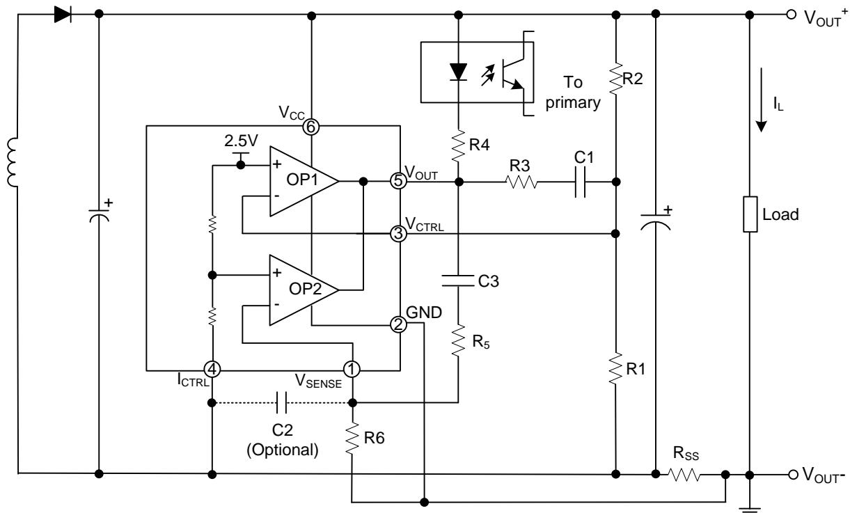
$$V_{OUT} = [V_{REF} + (I_L \times R_{SS})] \times \frac{R_1 + R_2}{R_1} - (I_L \times R_{SS})$$
