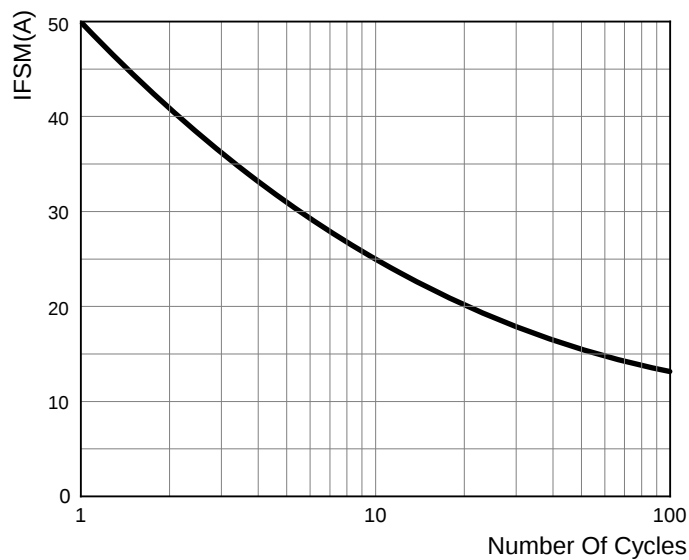
FIG 2: MAXIMUM NON-REPETITIVE FORWARD SURGE CURRENT
