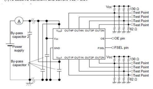
(2)To observe waveform and current Vcc = 2.5V
