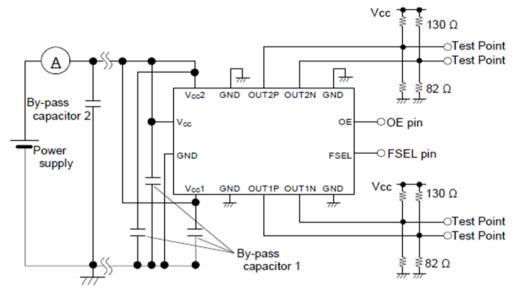
(2)To observe waveform and current Vcc = 2.5V
