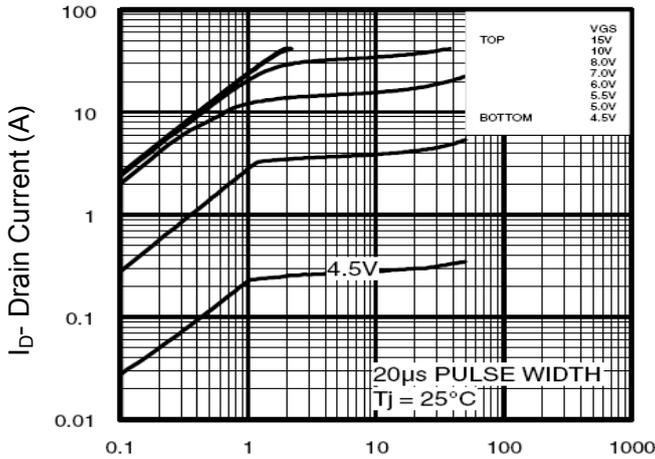
Figure 1 Output Characteristics
