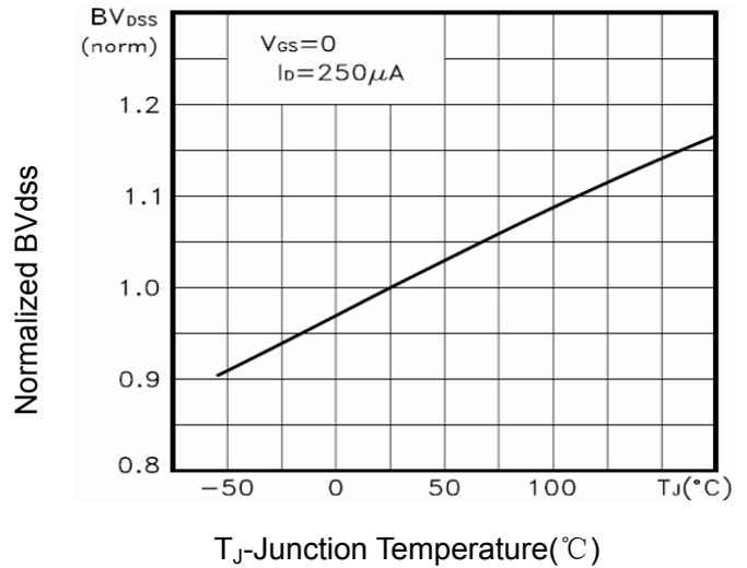
Figure 9 BV<sub>DSS</sub> vs Junction Temperature
