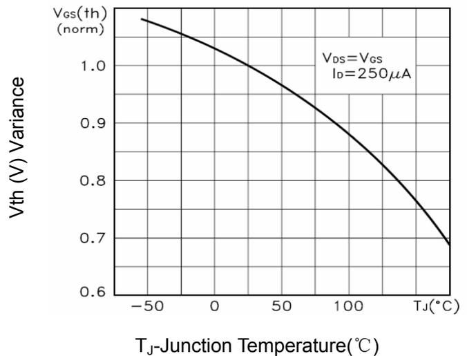
Figure 10 V<sub>GS(th)</sub> vs Junction Temperature
