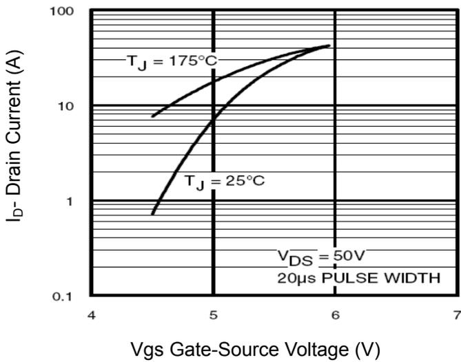
Figure 2 Transfer Characteristics
