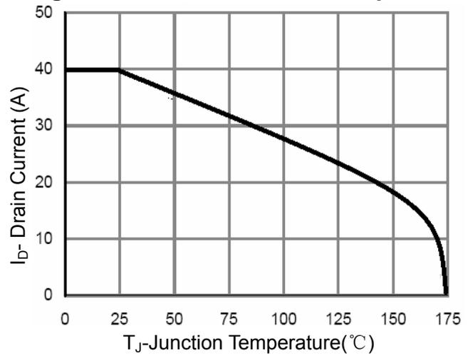
Figure 10  $I_D$  Current Derating vs Junction Temperature
