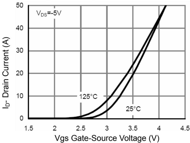
Figure 2 Transfer Characteristics
