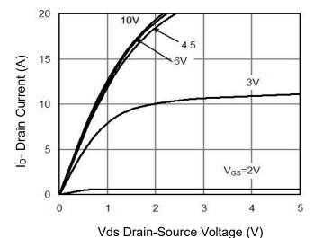
Figure 5 Output Characteristics
