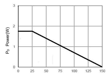
T<sub>J</sub>-Junction Temperature(°C) **Figure 3 Power Dissipation**
