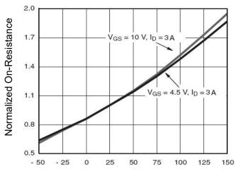
Figure 8 Drain-Source On-Resistance
