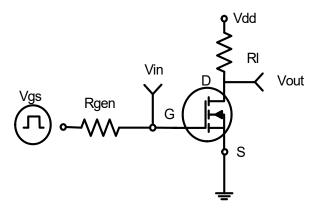
**Figure 1:Switching Test Circuit**
