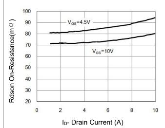
Figure 6 Drain-Source On-Resistance
