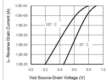
Figure 12 Source- Drain Diode Forward
