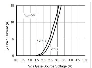
**Figure 7 Transfer Characteristics**
