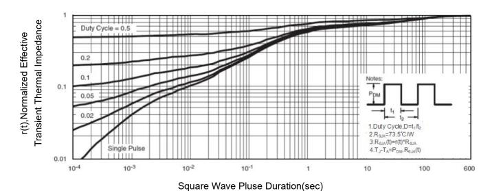
**Figure 14 Normalized Maximum Transient Thermal Impedance**
