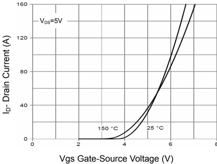
Figure 2 Transfer Characteristics
