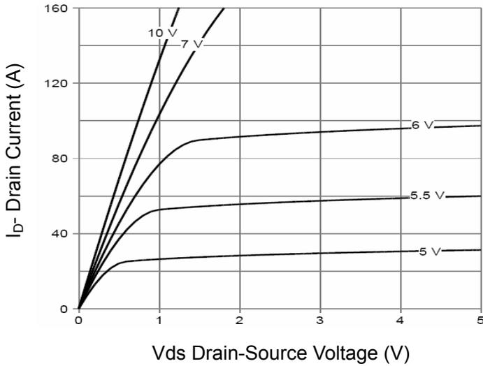
Figure 1 Output Characteristics
