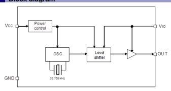
V<sub>IO</sub> is a power supply pin for OUT output and can also be used as an OE pin. Set V<sub>IO</sub> to 0 V when setting Disable.
