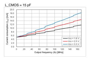
The actual current consumption is the total of the current under the condition of no load and the current to drive the output load (fo  $\times$  L\_CMOS  $\times$  V<sub>CC</sub>). To reduce the current consumption, it is effective to use lower frequency, lower supply voltage and lower output load.
