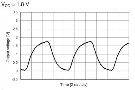
fo = 150 MHz, L\_CMOS = 15 pF, T\_use = +25 °C, Rise/Fall time: A (Default) or B (Faster)
