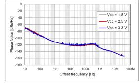
Phase jitter: 1.1 ps Typ. Offset frequency: 12 kHz to 20 MHz
