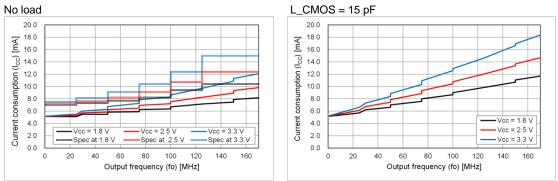
The actual current consumption is the total of the current under the condition of no load and the current to drive the output load (fo  $\times L_CMOS \times V_{CC}$ ). To reduce the current consumption, it is effective to use lower frequency, lower supply voltage and lower output load.
