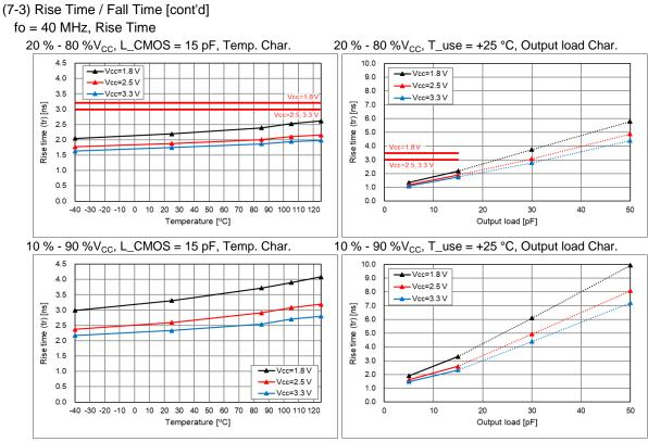
\* Output load condition under L\_CMOS > 15 pF (dotted line area) is not guaranteed, and the data is for reference.
