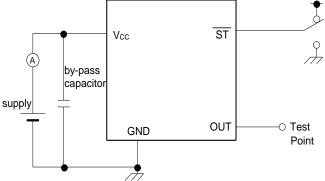
\*Standby current test should be  $\overline{ST} = GND$ .
