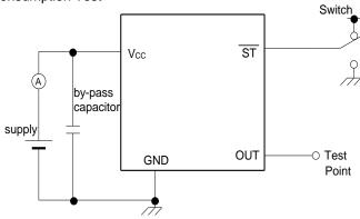
\*Standby current test should be  $\overline{ST} = GND$ .
