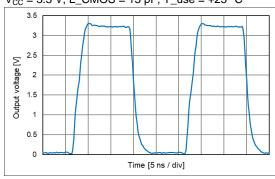
$V_{CC}$  = 2.5 V, L\_CMOS = 15 pF, T\_use = +25 °C
