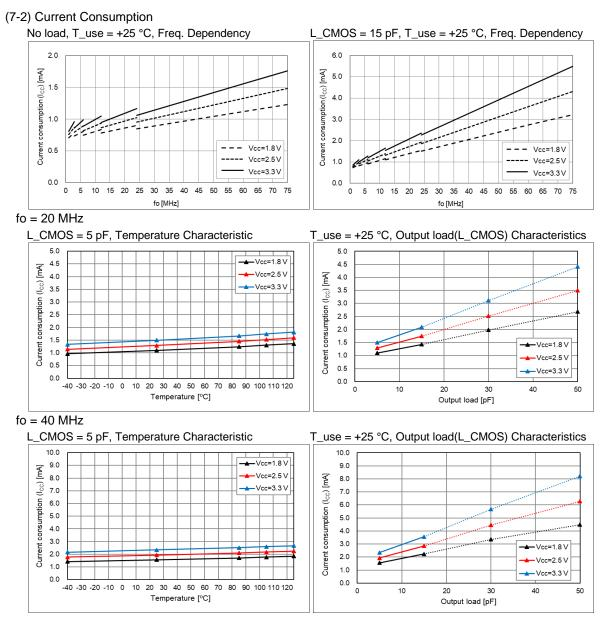
\* Output load condition under L\_CMOS > 15 pF (dotted line area) is not guaranteed, and the data is for reference. The actual current consumption is the total of the current under the condition of no load and the current to drive the output load (fo × L\_CMOS ×  $V_{CC}$ ). To reduce the current consumption, it is effective to use lower frequency, lower supply voltage and lower output load.
