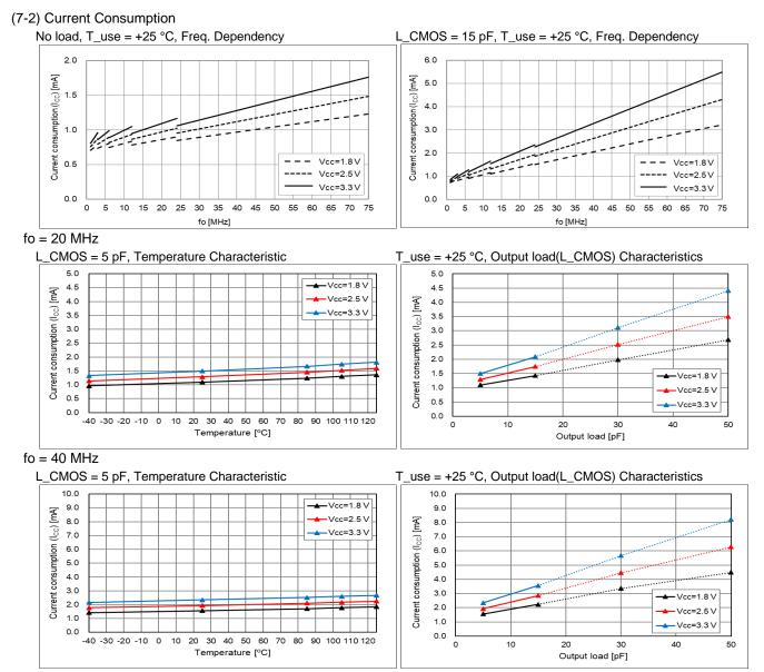
\* Output load condition under L\_CMOS > 15 pF (dotted line area) is not guaranteed, and the data is for reference. The actual current consumption is the total of the current under the condition of no load and the current to drive the output load (fo x L\_CMOS x V<sub>CC</sub>). To reduce the current consumption, it is effective to use lower frequency, lower supply voltage and lower output load.
