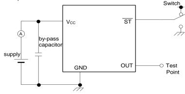
\*Standby current test should be  $\overline{ST} = GND$ .
