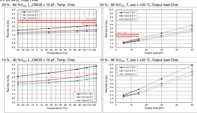
\* Output load condition under L\_CMOS > 15 pF (dotted line area) is not guaranteed, and the data is for reference.
