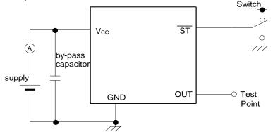
\*Standby current test should be  $\overline{ST} = GND$ .
