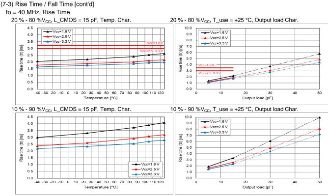
\* Output load condition under L\_CMOS > 15 pF (dotted line area) is not guaranteed, and the data is for reference.
