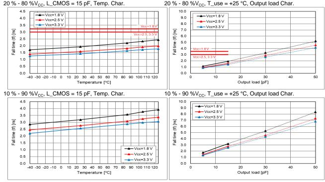
\* Output load condition under L\_CMOS > 15 pF (dotted line area) is not guaranteed, and the data is for reference.
