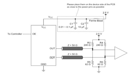
\* By-pass capacitor (approx. 0.01  $\mu$ F to 0.1  $\mu$ F) places closely between Vcc and GND.
