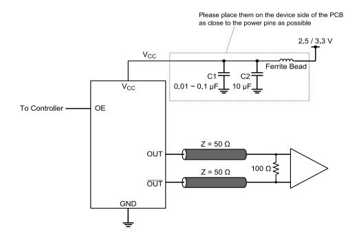
\* By-pass capacitor (approx. 0.01  $\mu$ F to 0.1  $\mu$ F) places closely between Vcc and GND.
