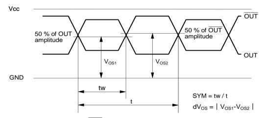
Differential output waveform (OUT –  $\overline{OUT}$ )
