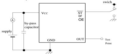
\*Current consumption under the disable function should be = GND.
