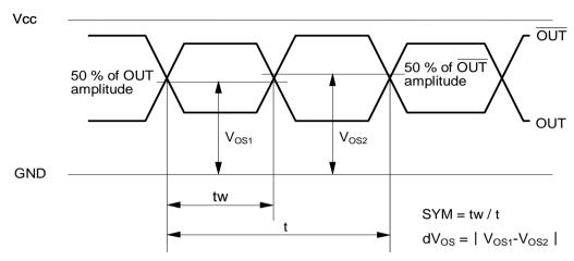
Differential output waveform (OUT - OUT)
