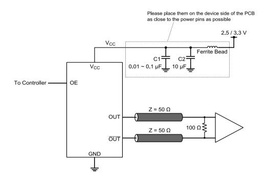
\* By-pass capacitor (approx. 0.01 µF to 0.1 µF) places closely between Vcc and GND.
