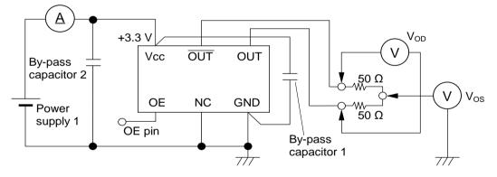
\* The lines from OUT and  $\overline{OUT}$  pin are same length.
