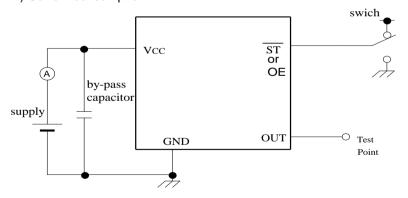
\*Current consumption under the disable function should be = GND.
