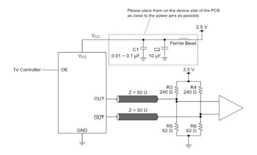
\* By-pass capacitor (approx. 0.01  $\mu$ F to 0.1  $\mu$ F) places closely between Vcc and GND.
