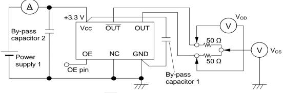
\* The lines from OUT and  $\overline{OUT}$  pin are same length.
