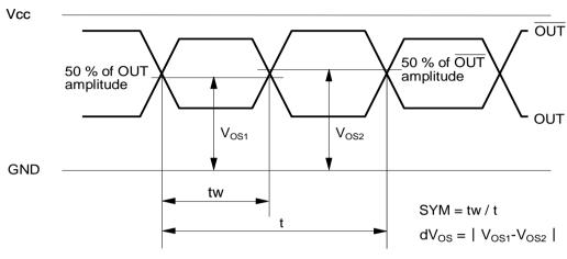
Differential output waveform (OUT - OUT)
