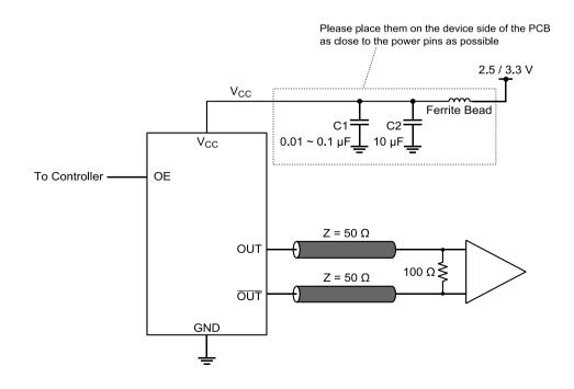
\* By-pass capacitor (approx. 0.01  $\mu$ F to 0.1  $\mu$ F) places closely between Vcc and GND. \* By-pass capacitor (approx. 10  $\mu$ F) places closely between power supply terminals on the board. \* Please design the two output lines by characteristic impedance 100  $\Omega$  and same length, and try to make the output lines as short as possible.
